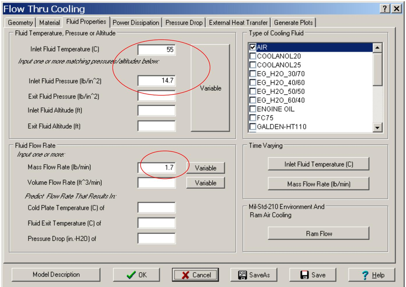
With the new model, fan curve is not include, just the flow rate at each condition. In this case and model, 1/2 the fan power is input.
