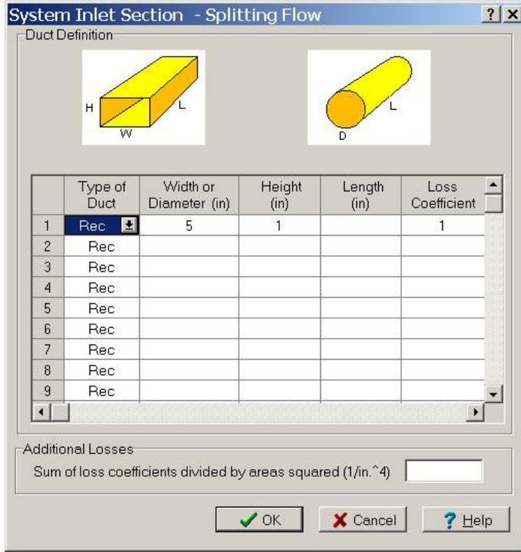
The "Inlet Section" geometry just prior to the cold plate is input here.
