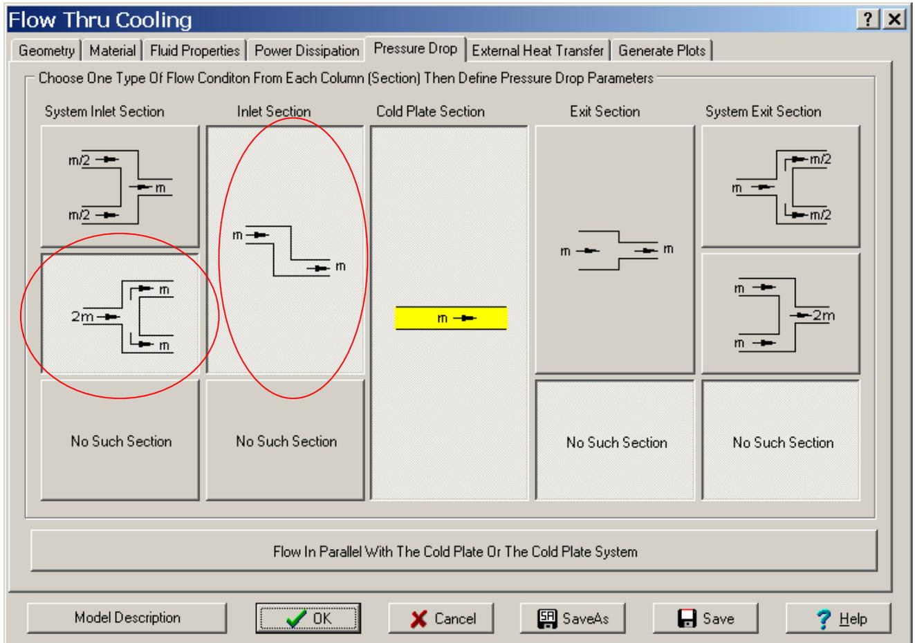
The "System Inlet Section" geometry at the fan is here.
